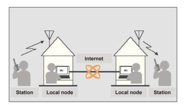
In addition to the WIRES features, WIRES-X also supports digital communications. Using WIRES-X, you can transmit and receive digitalized data such as text, image data and audio.
