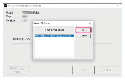
The firmware transfer starts and the FT5DR/DE firmware update executes (it takes about Main Firmware: 20 seconds or Sub Firmware: 90 seconds to complete the update). When the firmware update completes, a message appears.
