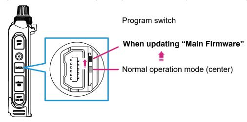
4. Use the supplied USB cable to connect the FT5DR/DE DATA jack to the computer.
