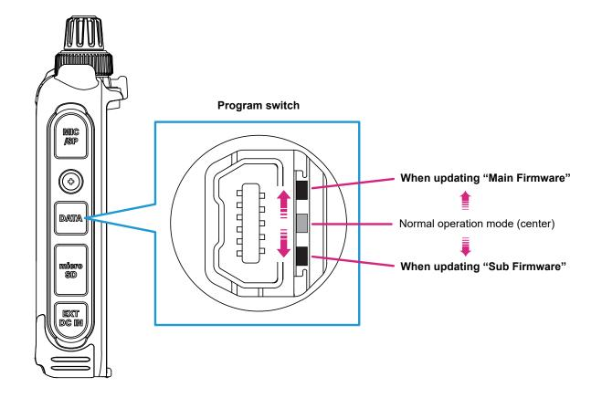
7. Use the supplied cable to connect the FT5DR/DE DATA jack to the computer.
