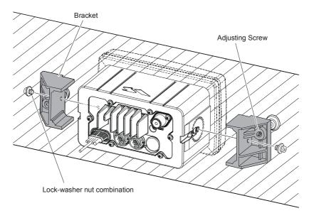
Figure 1. MMB-84 Flush Mount Installation
