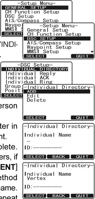
desired number and move one space to the right by pressing the [ENT] soft key. Repeat this procedure until all nine space of the MMSI number are entered.
