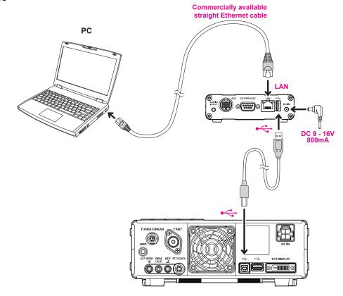
(3) Connection diagram for remote control within a local LAN using a router
