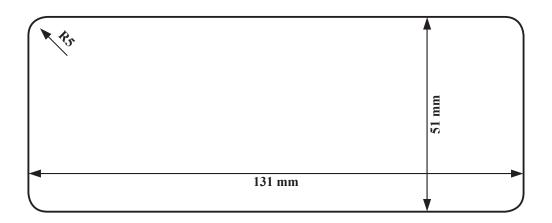
Use this template to mark the location where the rectangular hole for the flush mount is to be cut.
