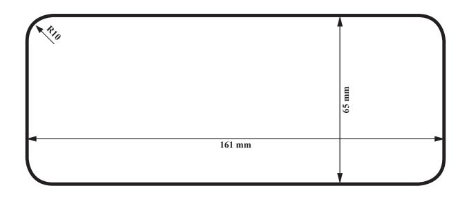
Use this template to mark the location where the rectangular hole for the flush mount is to be cut.
