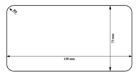
Use this template to mark the location where the rectangular hole for the flush mount is to be cut.
